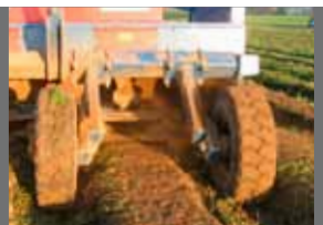
03 Hydraulically driven shakers for the separation of soil
